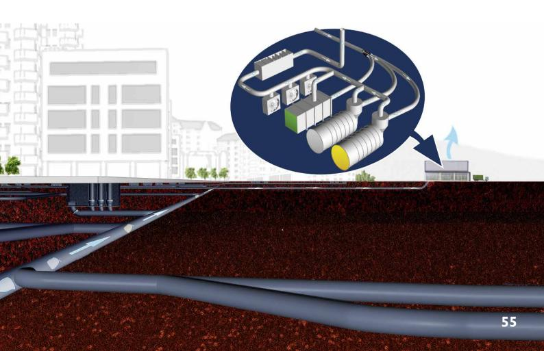
Figure 28: Vallastaden in Linköping where an innovative solution has been developed in the form of a culvert system for new infrastructure solutions. All cables/pipes – electric, optic fibre, district heating, sewage, water and a waste vacuum system - are placed in one large culvert which is 2.5 metres in diameter. The only system outside the culvert is the surface water system. With this solution the cable/pipe infrastructure takes up less space and is also 100 percent recyclable.48
